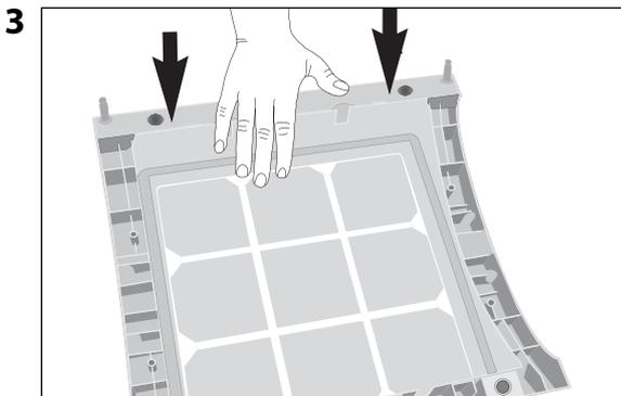
3 Press down until the mounting rail snaps into place. Repeat with second rail.
