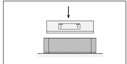
9. Turn the frame around and insert the new filter. Ensure that the arrows on the filter label point upward.
