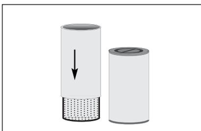
4. Pull a new filter sleeve over each new cartridge until it is completely covered.
