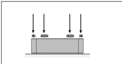
10. Make sure that the filter is inserted all the way into the frame. Insert the clamps into the sliding grooves inside the frame and push them down.
