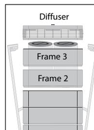
6. Replace frame 2 with the cartridges, frame 3 and the diffuser. Close the unit by pressing both arms together.
