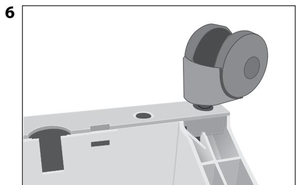
6 Ensure that each caster is securely fitted before placing the air purifier in its upright position onto the casters.
