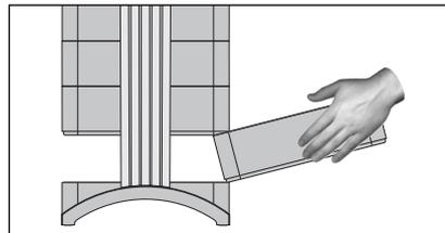
11. Put the frame back into the housing. For details on how to close the housing, please refer to the section 6.3.
