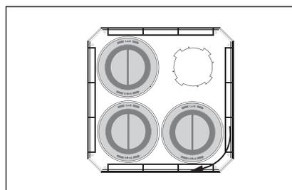
5. Insert the new cartridges in the base plate by turning the cartridge clockwise. Finally check that each cartridge is well secured in the base plate.
