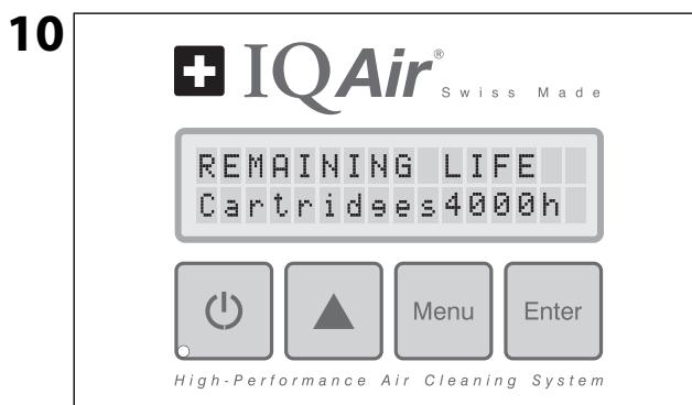
When used cartridges (or post-filter sleeves) have been replaced with a new set of cartridges (post-filter sleeves), the appropriate filter life monitor must be reset in the IQAir's control panel (please refer to the following paragraph).
