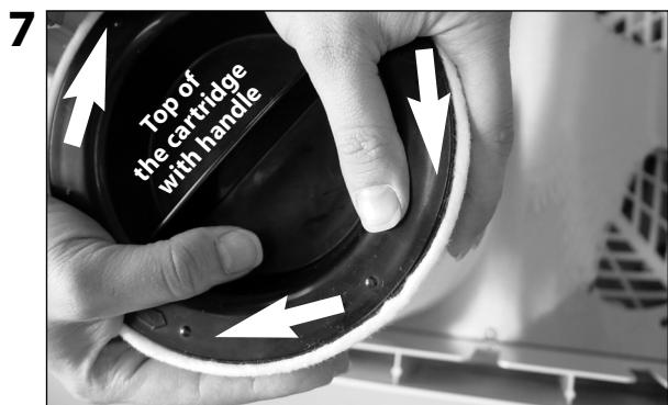
Once placed into the slots, turn the cartridge clockwise until it is securely locked onto the plate. Repeat with the remaining cartridges.
