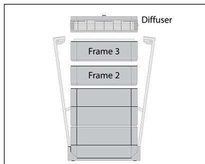
2. Opening the arms will release the top housing modules. Remove the diffuser and Frame 3. Then put these aside.
