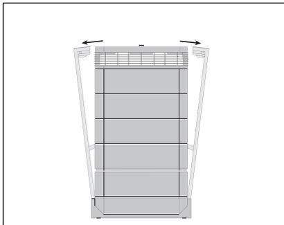
1. Open the locking arms, making sure they are fully extended outward. For details, refer to section 6.3.
