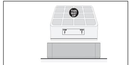
9. Turn the frame over (right side up again) and insert the new filter. Ensure that the arrows on the filter label point upward.
