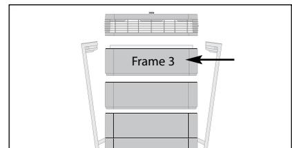
9. Put frame 3 back into the housing and reposition the diffuser. For closing refer to section 6.3.
