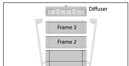
6. Put the frame back into the housing, followed by frame 3 and the diffuser. For closing refer to section 6.3.
