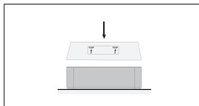
5. Insert the new filter. "TOP" indicates the filter's upright position. Ensure that "TOP" is visible when filter is installed.
