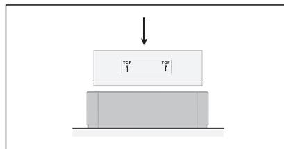
8. Turn the frame over (right side up again) and insert the new filter. Ensure that the arrows on the filter label point upward. The label “this way up” should be visible when installed properly. Re-install four filter clamps.
