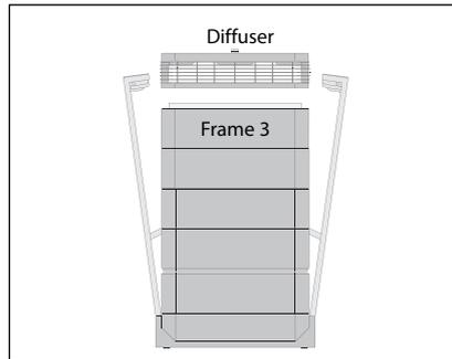
2. Opening the arms will release the top housing modules. Removing the diffuser will reveal the HyperHEPA filter inside Frame 3.
