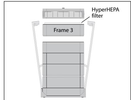
3. Remove Frame 3 containing the HyperHEPA filter.
