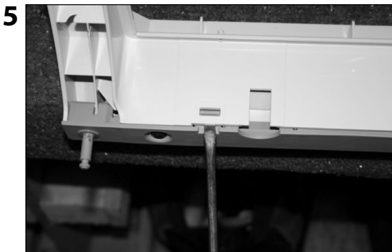
Using a flat-head screwdriver, press firmly into the slotted tab.
